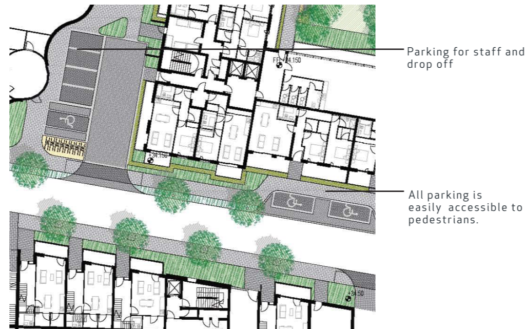
FIG 61 Plan view of street parking between Creche and Gym facility and Block A
